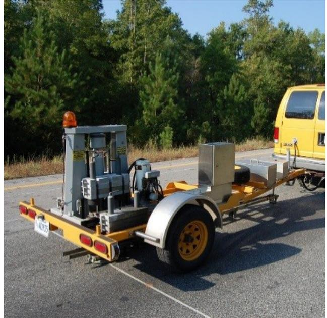
FWD, used in conjunction with pavement cores, provides a corroborated data set on which to determine the most appropriate and cost effective pavement rehabilitation treatment – which in many cases may be a combination of treatments due to varying pavement conditions throughout your corridor.
